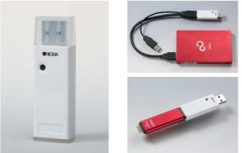
Figures 1-3, from left clockwise: Photo of *Enigma* module; the *Enigma* connected to a USB3.0/SATA hard drive; the *Enigma* connected to a USB2.0 Thumb drive. Enigma + USB MSC = Connected Pair
